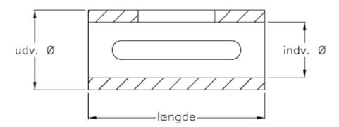
Description = 11/14Internal diameter = 11Length = 28Outer diameter = 14
